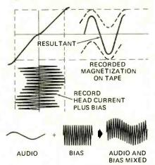
FIG. 9—COMBINING high-frequency bias with desired audio signals during recording shifts audio magnetization of tape to its linear undistorted region.
