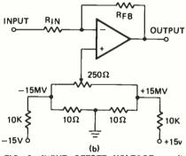
FIG. 3—INPUT OFFSET VOLTAGE results from a mismatch in the differential input stage. Two methods for reducing the voltage is shown.
