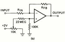
FIG. 4—INPUT OFFSET CURRENT results from a mismatch in the input stage. Two methods for reducing the current is shown.
