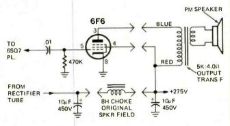
pin 3, and screen-grid, pin 4, of the 6F6. That 10-µF electrolytic capacitor should also go to the screen.
