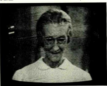
FIG. 3—HERRINGBONE PATTERN usually caused by FM interference.
