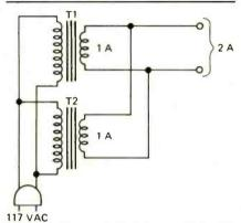
FIG. 4—A CURRENT-BOOSTING HOOKUP. Identical transformers give the best results.
