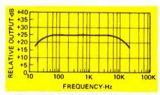
FIG. 6—COMBINING RECORDING RE-SPONSE (Fig. 2) with equalized playback response (Fig. 5) results in overall record/ play response shown.
