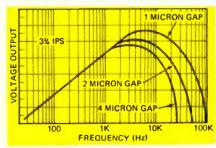
FIG. 4—REDUCING PLAYBACK HEAD GAP while maintaining constant tape speed will extend the high-frequency response.
