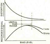
FIG. 10—INCREASING BIAS LEVEL reduces distortion, but overbiasing will reduce high-frequency response.
