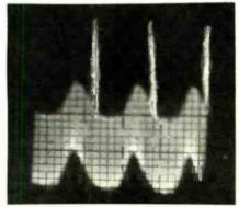
FIG. 2—VERTICAL SPIKES appear among hash at the terminal of one of the filter capacitors in the power supply.
