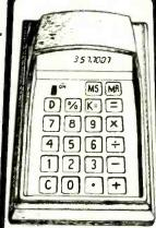
5 function (+ - x ÷ %) plus separate memory and constant registers. Floating point, 8 digit, timed display turnoff, low battery indicator. Kit complete with instructions, all parts, and handsome gray case, but less batteries.
