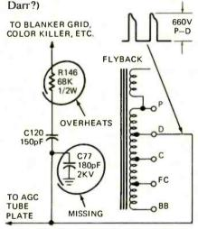
In circuits with high pulse voltages, an open bypass can cause this. The bypass capacitor reduces the amplitude of the pulse, so that the resistor can hold. Good suspect would be C77, 180 pF, which is right on the flyback terminal board. You might overlook this, because it's drawn on the schematic away up on the age tube plate!
