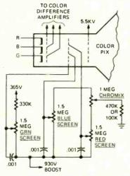
The diagram shows the screen control circuit of this one, which is a voltage divider between B+400 volts and B++950 volts. You obviously have the boost-boost voltage on these controls; it looks very much as if the circuit to B+ 400 volts is open. Check; you should be able to get those screen voltages down to around +400 volts. If you can't, find out why.
