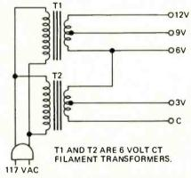
FIG. 3—ADJUSTABLE-VOLTAGE UNIT, using two center-tapped 6-volt transformers.
