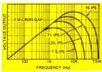
FIG. 3—LINEAR INCREASE IN OUTPUT VOLTAGE extends to higher frequencies at increased tape speed.
