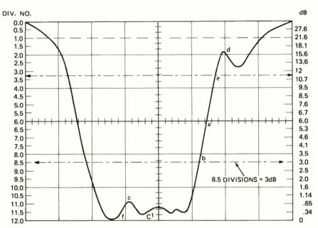
DECIBELS MAY BE MEASURED QUICKLY and with reasonable accuracy by using an oscilloscope with the simple scale shown. No calculation is necessary. Each vertical graduation on the figure, which normally represents one centimeter, has been subdivided into four divisions. On the left side are the division numbers and on the right the corresponding value of each division in decibels.
