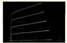
FAMILY OF CURVES FOR A H1GH-GAIN silicon pnp transistor (MPS-6522). Curve tracer settings are: step generator, 0.005 mA/step; collector series limiting resistance, 1000 ohms; horizontal sensitivity, 4 volts/cm; vertical sensitivity, 1 mA/cm. At 8 volts Vcs and an average collector current of 3.5 mA, beta is calculated to be 1.45 mA/0.005 mA, or 290.
